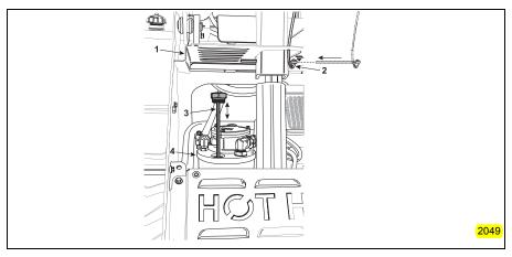
Figure 4-4 Hydraulic Fluid Level Dip Stick
